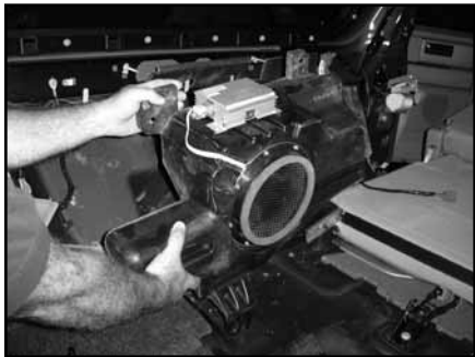
STEP 22 Remove the woofer system from the SUV.
